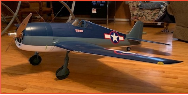
Tony Eck shows off his Top Flight Hellcat F6F. It has an 86 inch wingspan, and weights 27 lbs 10 ozs ready to fly. Its powered by a 12 cell battery pack with a Scorpion motor 4300 watts and swings a 26x12 prop.
