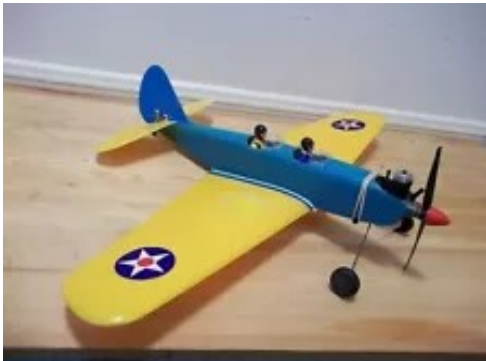
Pictured above is a Cox PT19. The idea of this plane was that the engine, landing gear and wing were held in place with rubber bands, for better crash resistance.
