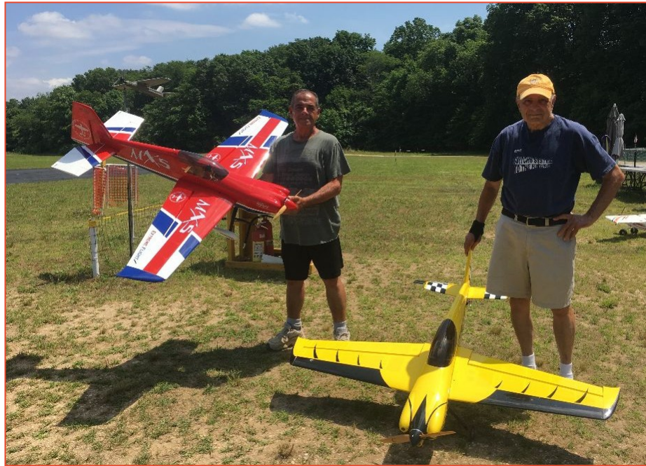
Tony C and Armand show off their new Extreme Flight MXS aerobatic planes with different color schemes. They have a 64 inch wingspan and use a 6S sized battery.
