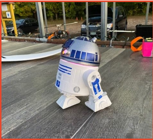
R2D2 made a special appearance at the field. He is a radio controlled 3D printing project created by Kevin Techner. The animated robot stands about 12 inches tall and has working lights, and maneuvers very well. Very impressive.
