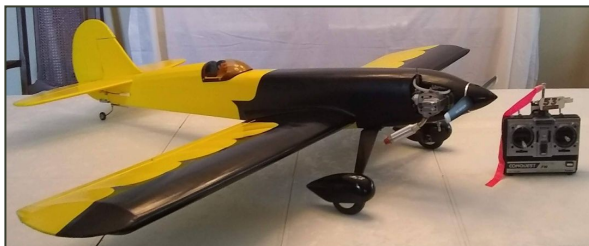
Great Planes Super Sportster 60, with OS 90-4 stroke, wing span of 60" Futaba radio 4 channel radio/FM, 5 servos, covered in 21 century covering.
