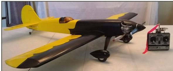
Great Planes Super Sportster 60, with OS 90-4 stroke, wing span of 60" Futaba radio 4 channel radio/FM, 5 servos, covered in 21 century covering.
