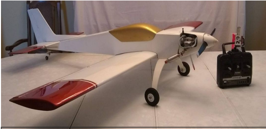
Goldberg Tiger 2, 61" wingspan, OS70-4 stroke, 5 servos, Futaba radio, 5 channel, Additional 2 gal glow fuel, glo plugs.
