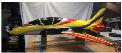
In the picture above, is a HSD v2 EDF 105mm jet that Dennis did some modifications to as well as repaint. It has an upgraded EDF fan replaced all HSD control system with FrSky control board, and its now a 12 channel. Mursier set up 2 receivers for redundancy and 12s battery packs.
