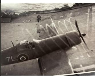
The photo on the left is a picture of a Corsair on an aircraft carrier. The moisture in the air clearly shows the **prop wash** caused by the prop. This is one of the forces created by the prop as it bites into the air. The *torque* of the prop causes the plane to want to go to the left. It is also referred to as the P-factor. "Be ready with the rudder".
